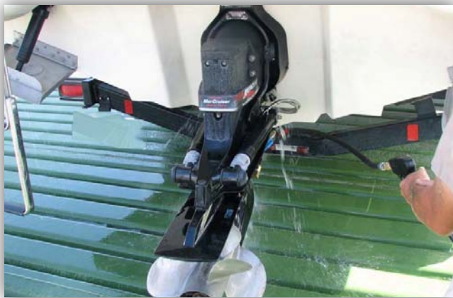
Invasive species can become trapped in watercraft engines and transported to new locations. Proper engine flushing is recommended to prevent future invasions (Photo credit: Bureau of Reclamation).
