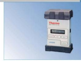
The Thermo Scientific personal DataRAM pDR-1000AN Monitor is a passive sampling, light-scattering nephelometer that measures real-time mass concentrations of dust, smoke, mists, and fumes in industrial as well as other indoor and outdoor environments.
