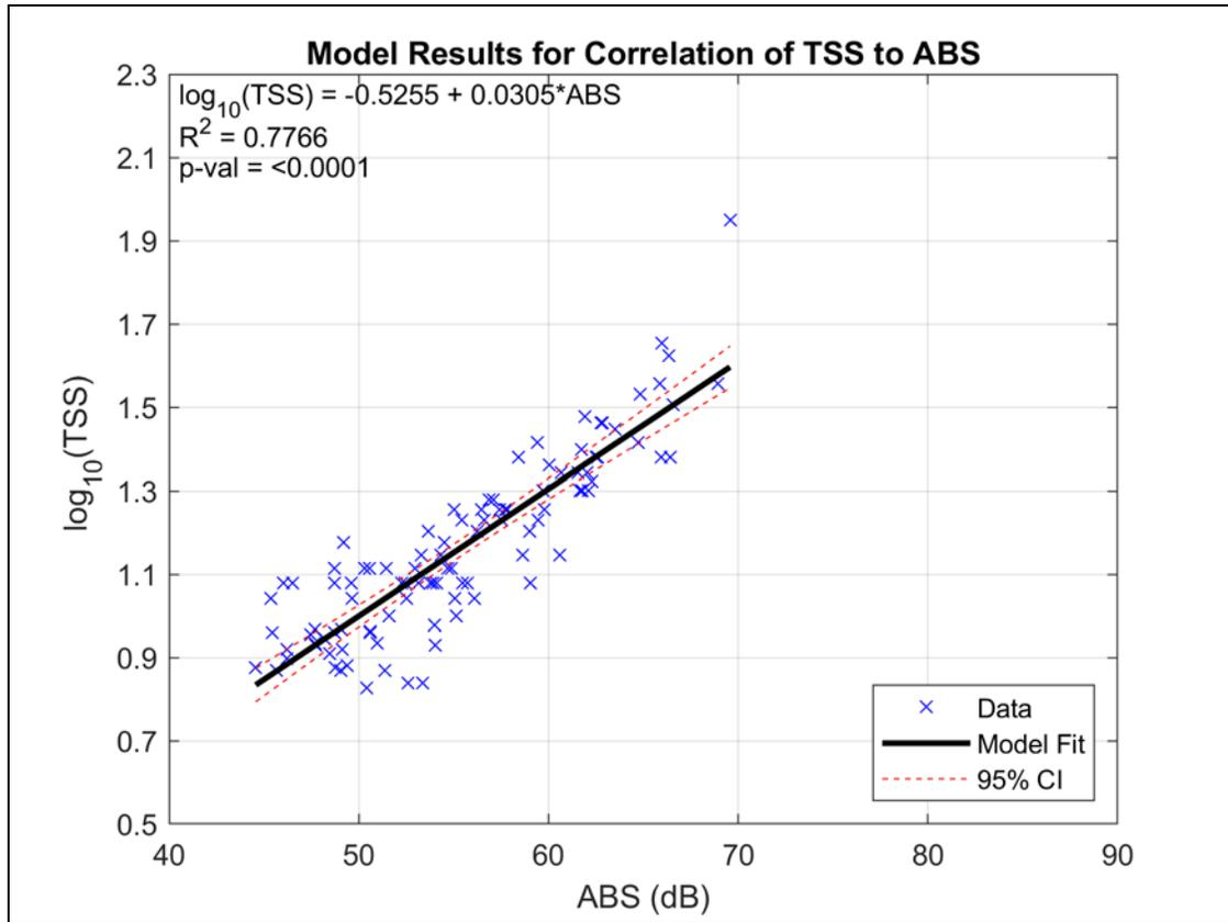
**Figure 4-2.** Calibration curve from linear regression analysis for TSS to ABS, plotted on increased scale to illustrate levels observed during the trials relative to the WQC standards for the Hudson River.
