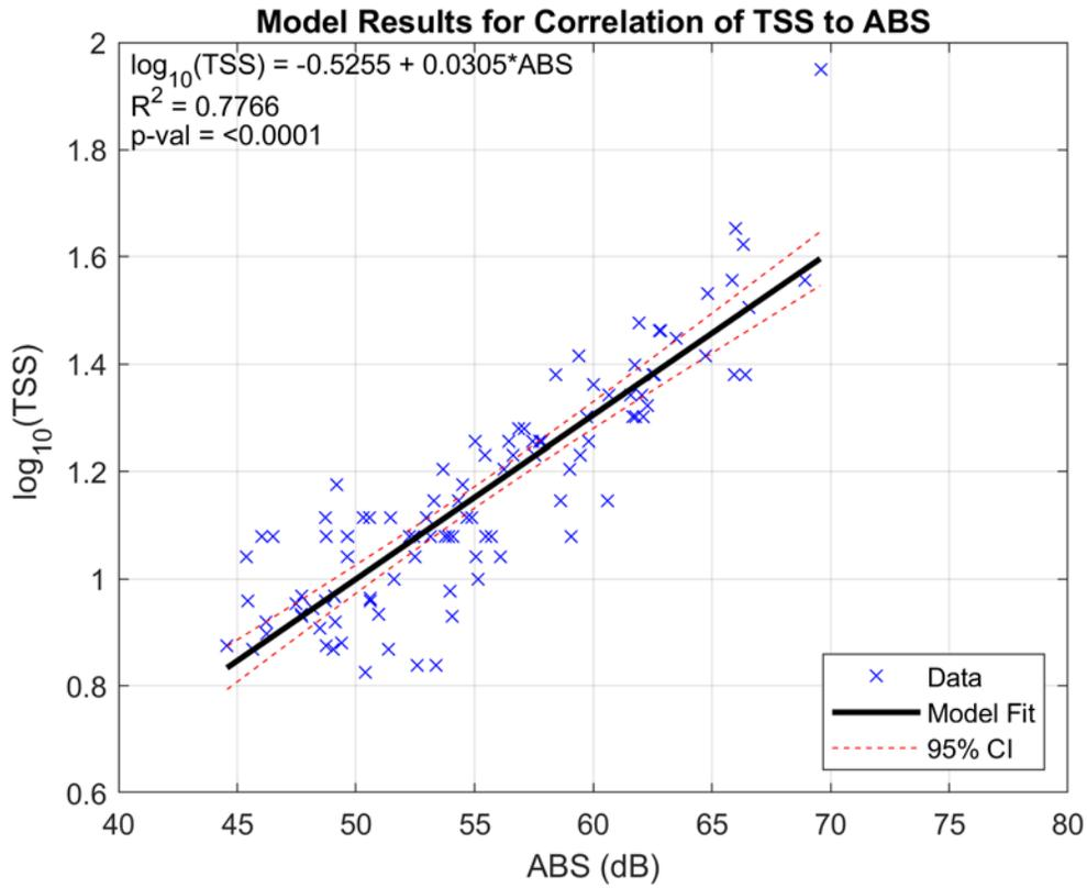
**Figure 3-5.** Calibration results for the linear regression analysis of  $\log_{10}(\text{TSS})$  to ABS for paired sample data (N = 102) collected from the Hudson River trial (9-Sep-2022) and the ambient river survey (7-Sep-2022).
