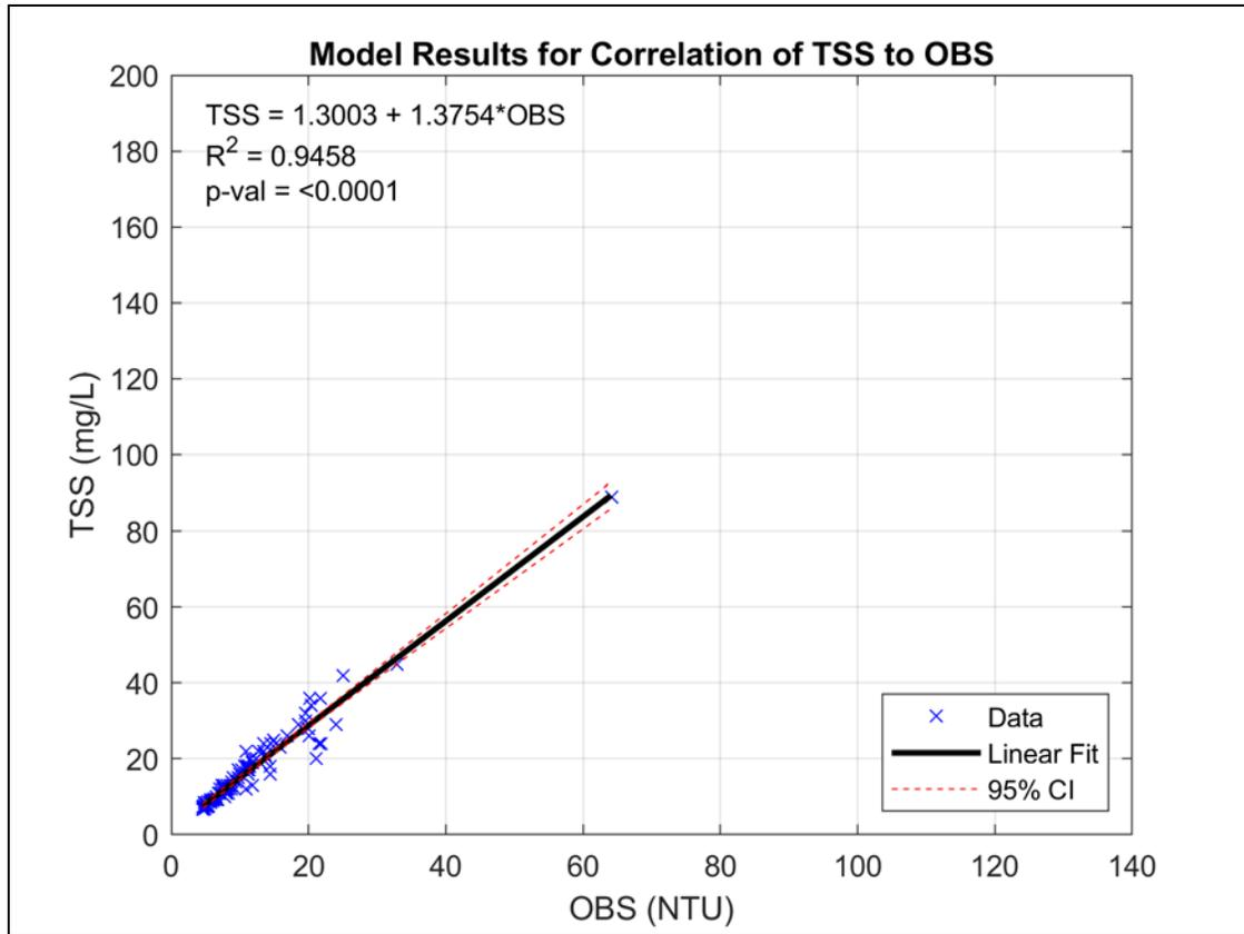
**Figure 4-1.** Calibration curve from linear regression analysis for TSS to OBS, plotted on increased scale to illustrate levels observed during the trials relative to the WQC standards for the Hudson River.
