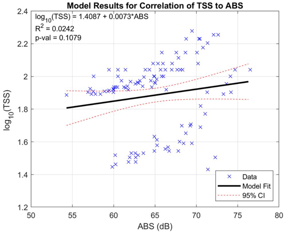
**Figure 3-5.** Calibration results for the linear regression analysis of  $\log_{10}(\text{TSS})$  to ABS for paired sample data (N = 108) collected from the Hudson River trial (22-Dec-2023) and the ambient river survey (22-Dec-2023).
