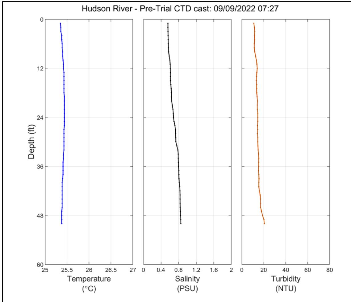
**Figure 3-1. CTD-OBS profiles of temperature, salinity, and turbidity (OBS) from Hudson River site prior to of the jet plow trial near the end of ebb tidal stage.**
