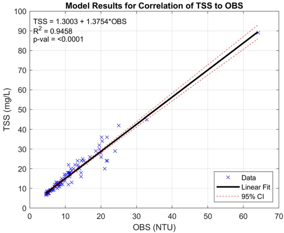
**Figure 3-4.** Calibration results for linear regression analysis of TSS to OBS for all paired sample data (N = 102) collected from the Hudson River trial (9-Sep-2022) and the ambient river survey (7-Sep-2022).
