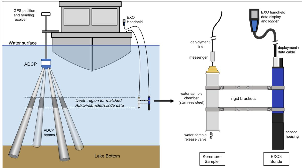
**Figure 2-1. Sampling equipment schematic diagram showing the relative deployment positioning of the ADCP, CTD-OBS, and Kemmerer sampler with respect to the vessel and water column on the left-hand side. To the right is a zoomed diagram of the design of the CTD-OBS-Kemmerer mount used during TSS monitoring.**
