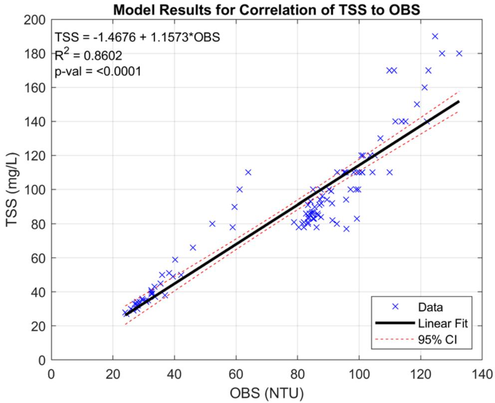
**Figure 3-4.** Calibration results for linear regression analysis of TSS to OBS for all paired sample data (N = 108) collected from the Hudson River trial (22-Dec-2023) and the ambient river survey (19-Dec-2023).
