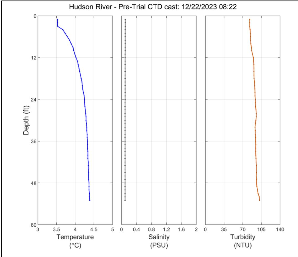
**Figure 3-1. CTD-OBS profiles of temperature, salinity, and turbidity (OBS) from Hudson River site prior to of the trencher trial during flood tidal currents.**
