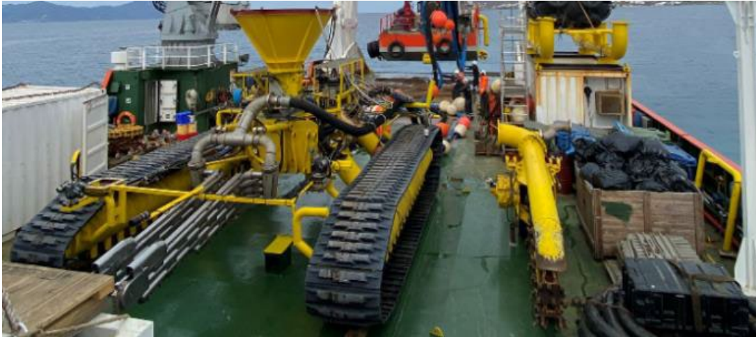
Figure 5-5 Remedial Burial Tool
