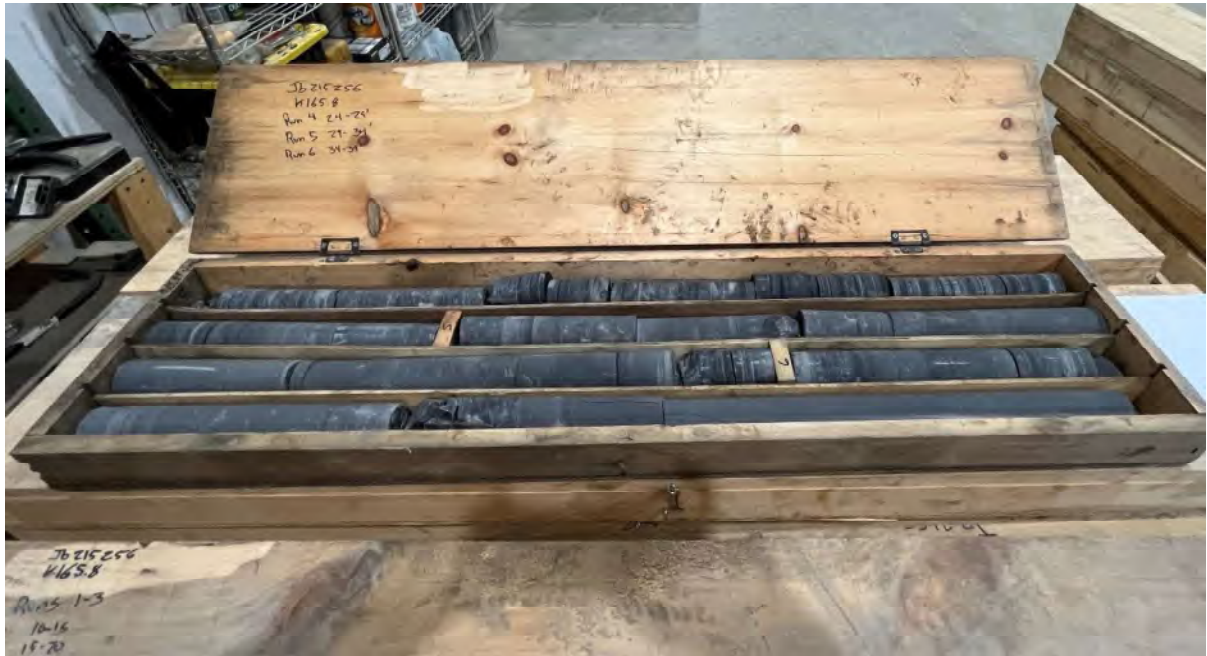
Rock Core – Boring K-165.8 (Runs 4-6)
