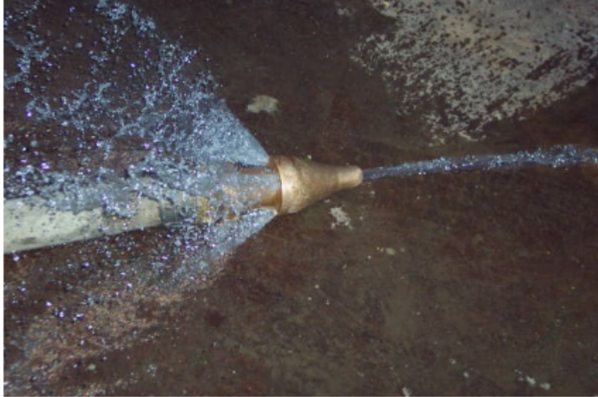
Figure 20-'Navy type' reactionless jet nozzle (diver operated)
