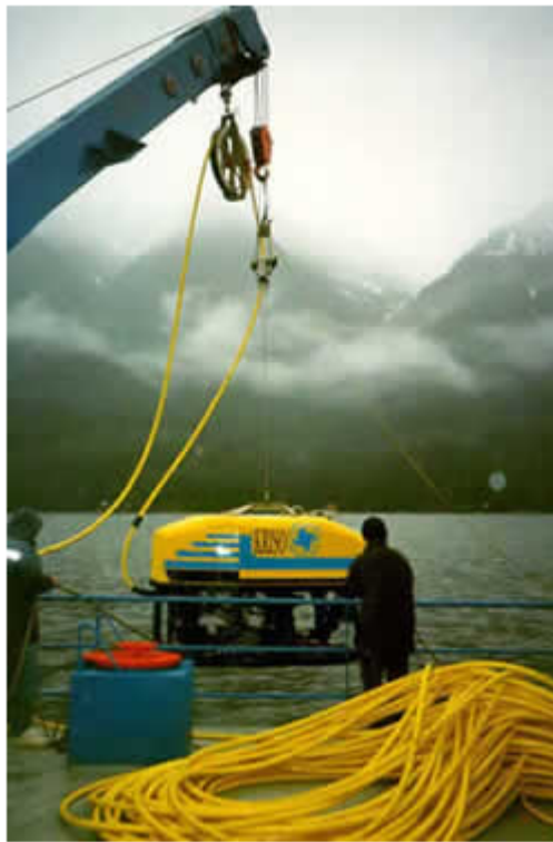
Figure 12 - Typical TDM ROV – Large Observational Class
