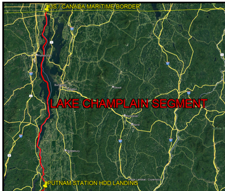
Figure 1 - Lake Champlain Submarine Cable Installation Segment
