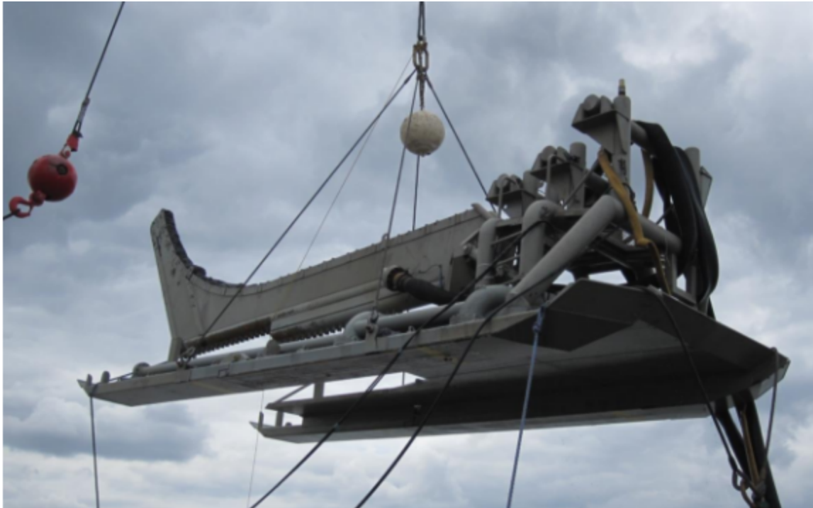
Figure 23 – ETA Jet/Shear Plow Sled (Typical)
