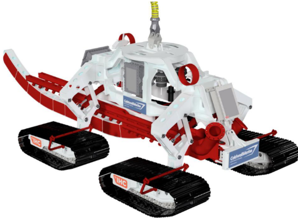
Figure 18 - Post-Lay Protection – Jetter Vehicle (Typical)
