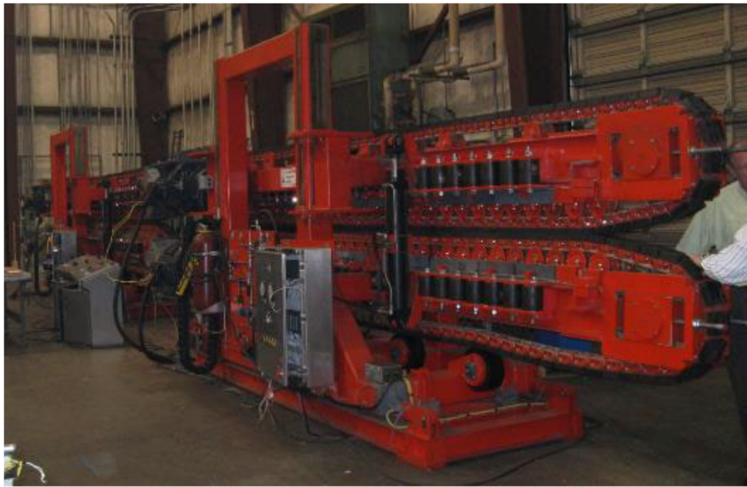
Figure 10 – Linear Cable Engine -typical (LCE)
