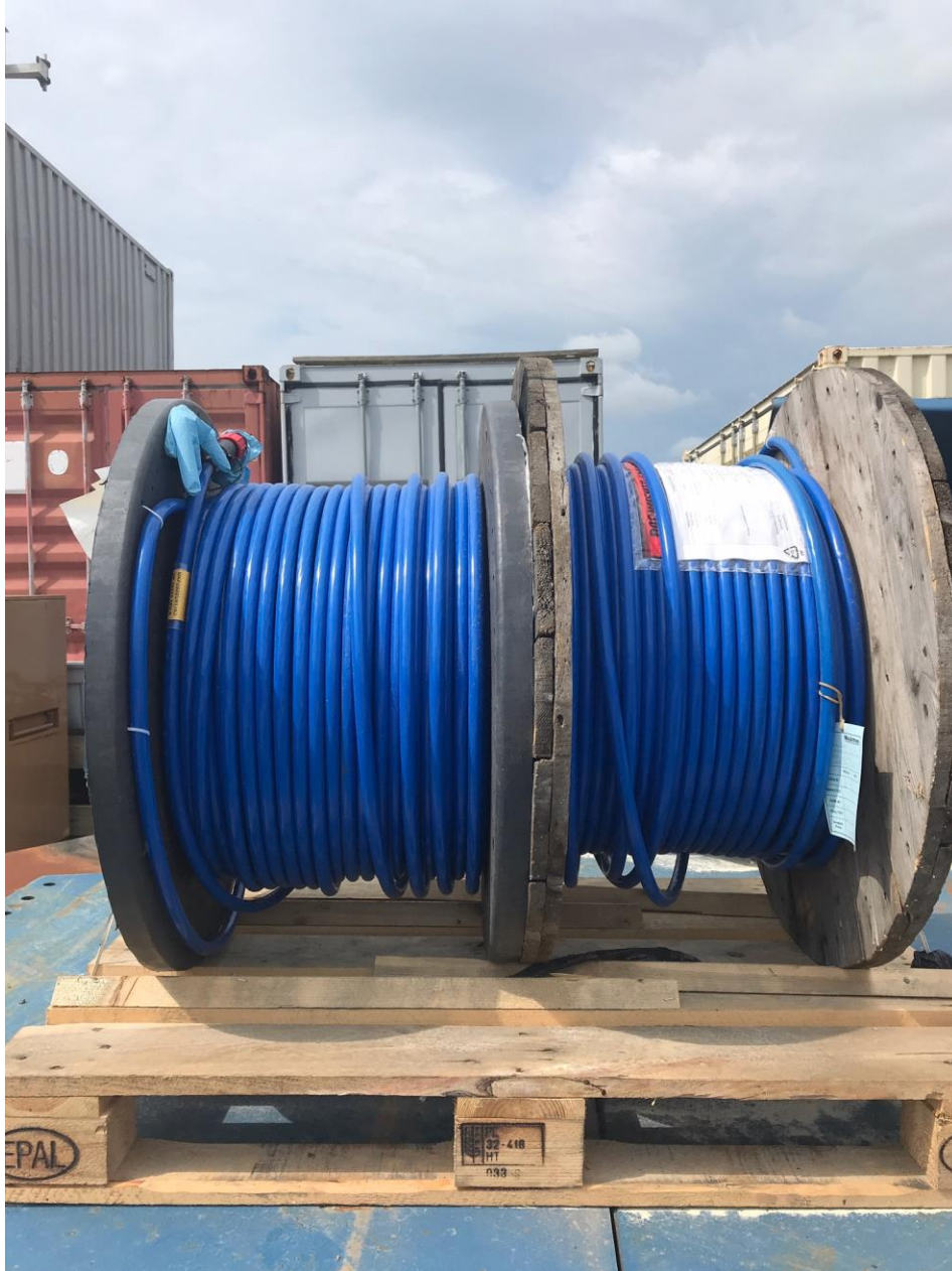
Figure 1 - Plow Umbilical (Primary + Spare)
