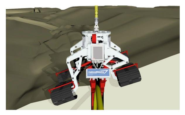
Figure 2 - Hi-Traq Jetter, Surface Fed, Amphibious – Trenching over challenging terrain
