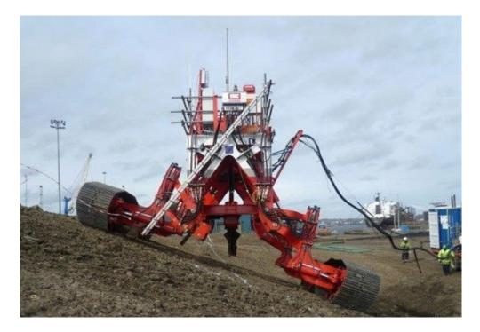
Figure 5 - Track Self-Levelling
