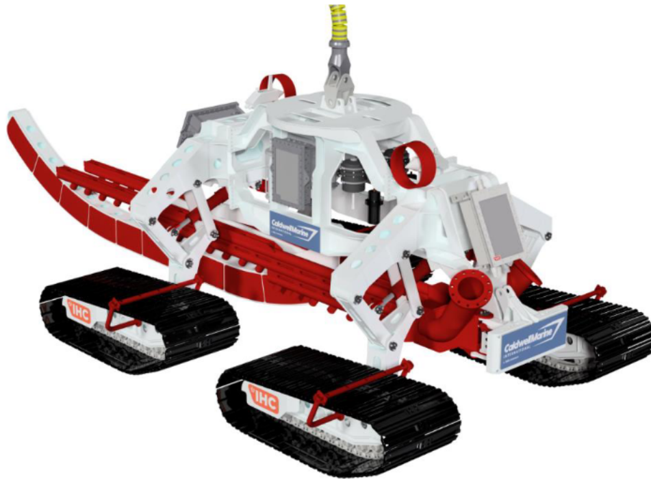
Figure 18 - Post-Lay Protection – Jetter Vehicle (Typical)
