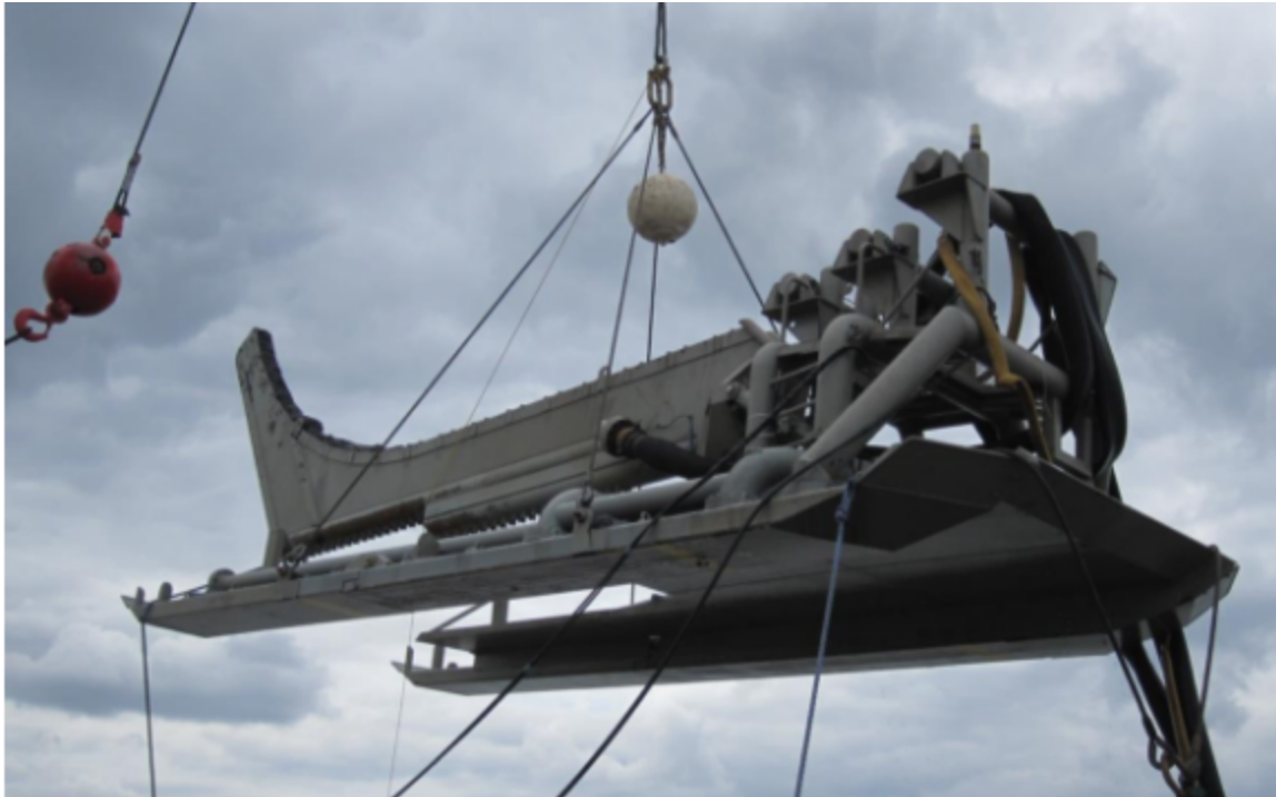
Figure 23 – ETA Jet/Shear Plow Sled (Typical)
