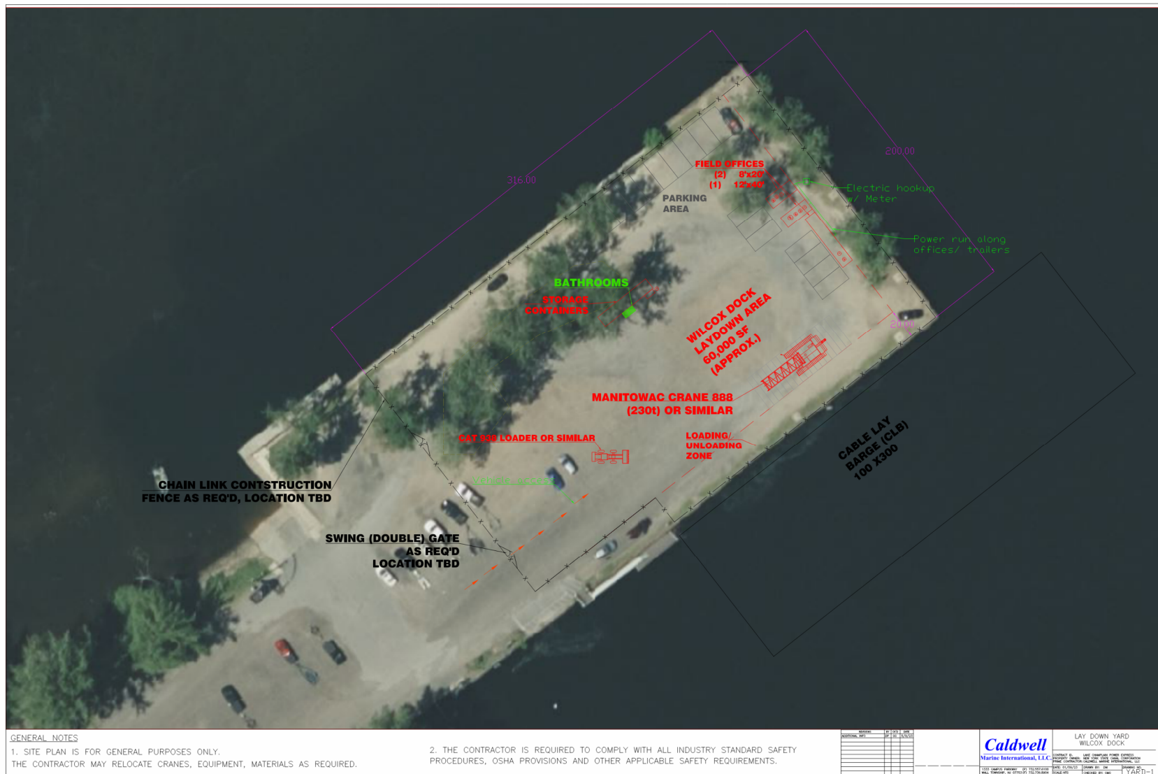
Figure 7- Wilcox Dock Yard Layout Schematic, Plattsburgh, New York
