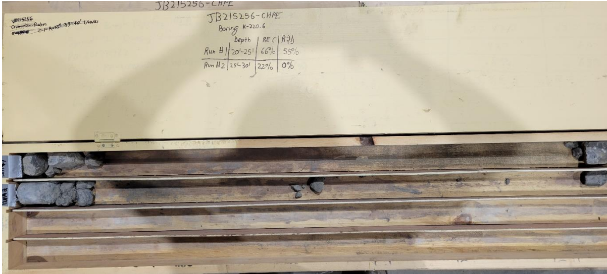
Rock Core – Boring K-220.6 (samples pulled for testing)
