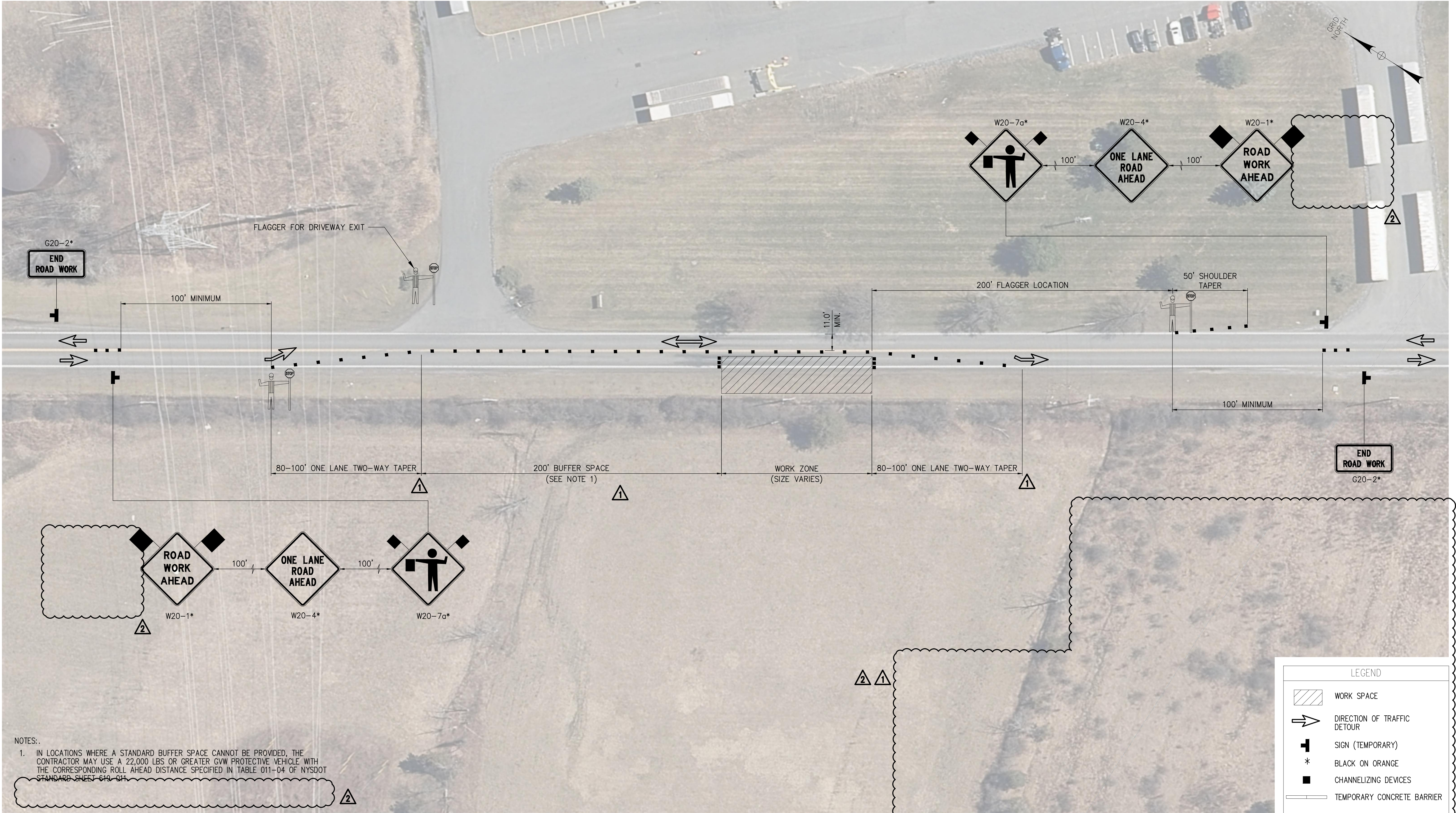
FLAGGER OPERATION, SHORT/INTERMEDIATE TERM STATIONARY, ONE LANE CLOSURE ON WEST YARD ROAD SCALE: 1" = 30'
