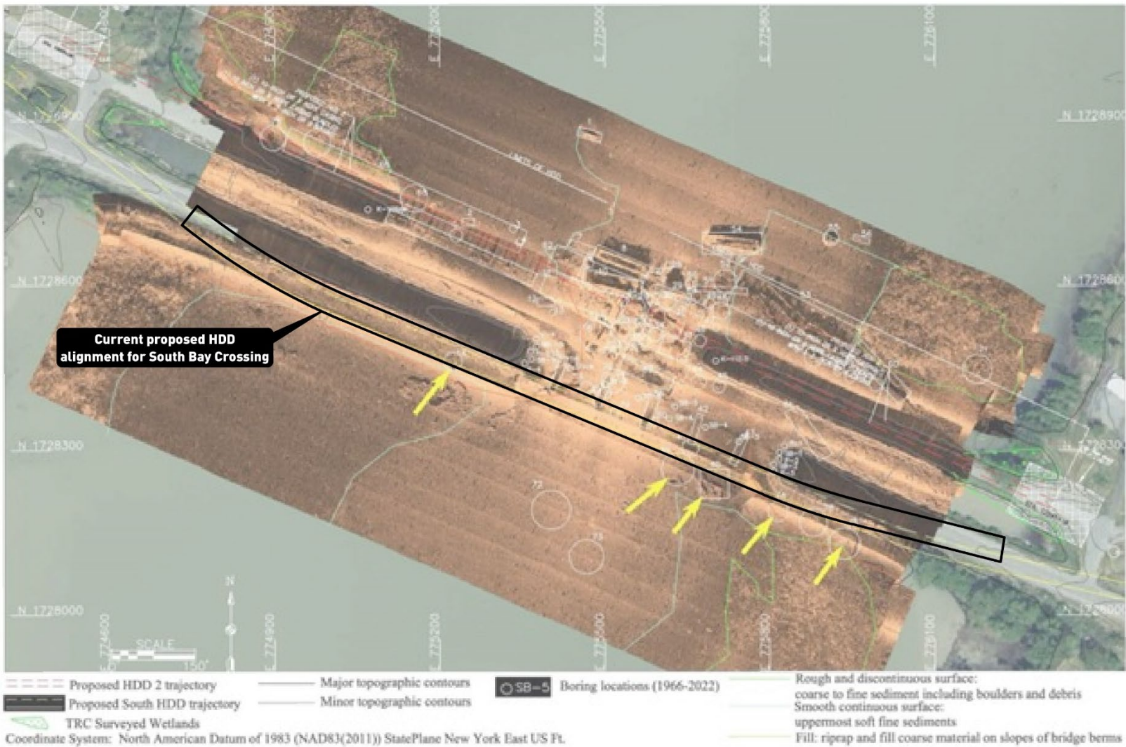
Figure 3: Side scan sonar and magnetometer targets identified near the southern HDD alignment indicated with yellow arrow (modified from Schnabel Geophysical survey report, 2022).
