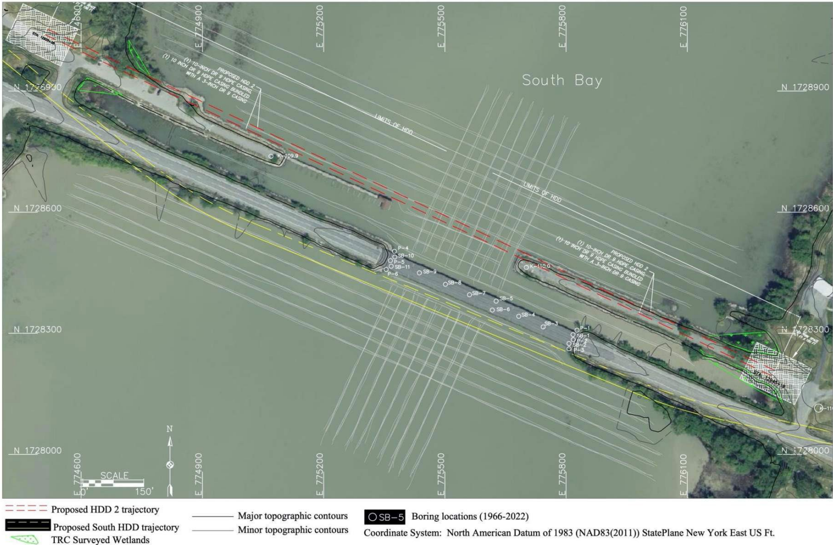
Figure 1: Aerial photograph of the project area with both proposed HDD alignments depicted. The northern alignment in red and the southern in yellow. (modified from Schnabel Geophysical survey report, 2022).
